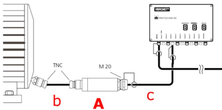
A: Junction box for one sensor cable VIB 6.770/13 (mounted electrically insulated)
