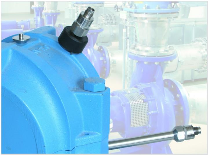
Mounting options for an "industrial" accelerometer
