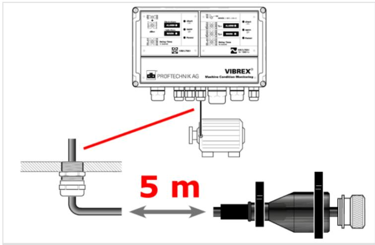
VIBREX sensor cable, 5-meter long.
