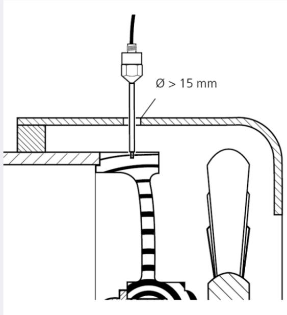
! : No contact between the extension rod and cover.
